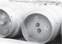
Photo 4. View of the access valves of the small HFC-134a–containing cylinder.
