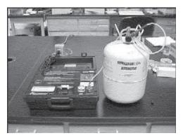
Refrigerant identifiers/analysers are small portable units used to identify certain ODS and non-ODS<sup>1</sup>. The more sophisticated models detect CFCs, HCFCs, HFCs and hydrocarbons. They are also able to analyse the composition of certain refrigerant blends, water content, and purity and to indicate the presence of highly flammable substances. Some manufacturers of refrigerant identifiers (for illustrative purposes only) are Bacharach, Neutronics, Robinair and Yokogawa.
