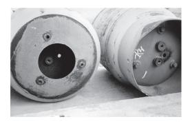
Photo 1. The access points to the main CFC-12 container become visible only after the double-layered container is cut open.
