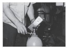
Photo 3. Example of leak detector.
