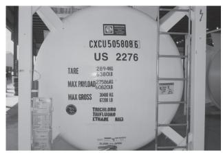
Photo 17 - Front end of an ISO tank (see box for example of ISO tank labelling).
