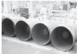
Photo 2 . View of the smallHFC-134a cylinders after removing the CFC-12 refrigerant and cutting open the main containers.
